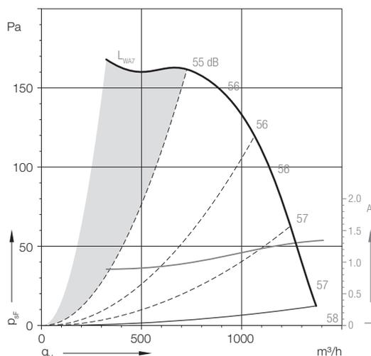
For a proper fan selection the duty point in the grey area to the left of the leftmost dashed parabolic line drawn on each performance diagram should preferably be avoided. In this area the fan stall is producing fluctuating pressure and fluctuating loads on the fan and motor; some single-phase motors may also be overheating in this low-load condition.
