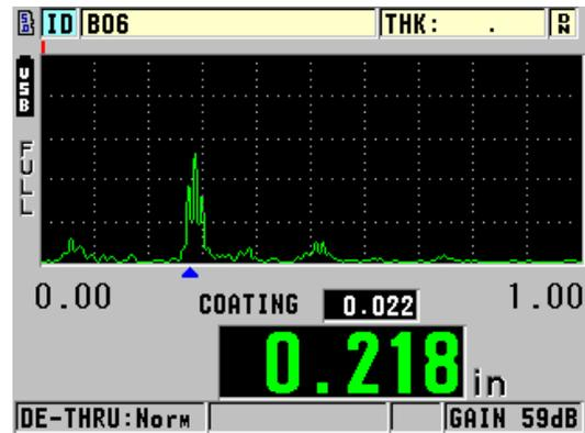
THRU-COAT mode with optional waveform
