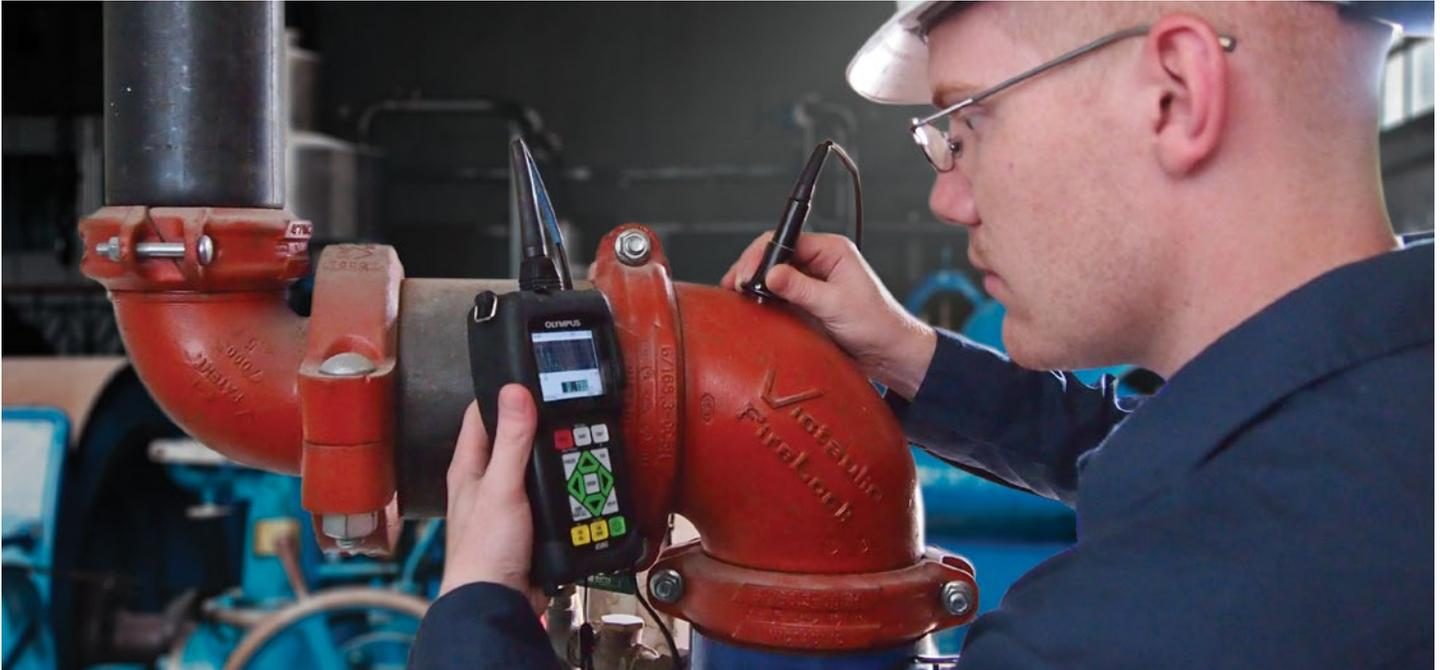
The 45MG is an advanced ultrasonic thickness gage packed with standard measurement features and software options. This unique instrument is compatible with the complete range of Olympus dual element and single element thickness gage transducers, making this innovative instrument an all-in-one solution for virtually every thickness gage application.
