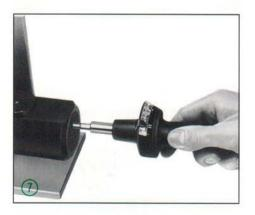
b) Position TORSIOMETER and apply required force (see 3.) (the trailing pointer will follow the pointer) ③.
