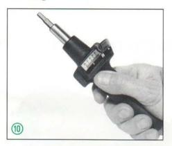
c) Before reusing the tool, slide the trailing pointer back to the starting position (see 4.3a).
