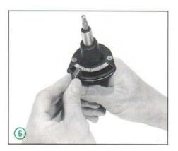
**4.3** Recording the torque applied in Ncm (only for clockwise use).
