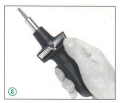
After the pressure is released, the trailing pointer will remain below the reading previously attained (10).
