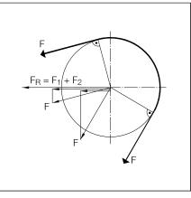
For measuring purposes, only those components, i.e.  $F_1$  and  $F_2$  effective in the direction of measuring, are relevant. The resultant measuring force is the sum of  $F_1 + F_2$ . This is halved, given centred web travel, between the two load cells.
