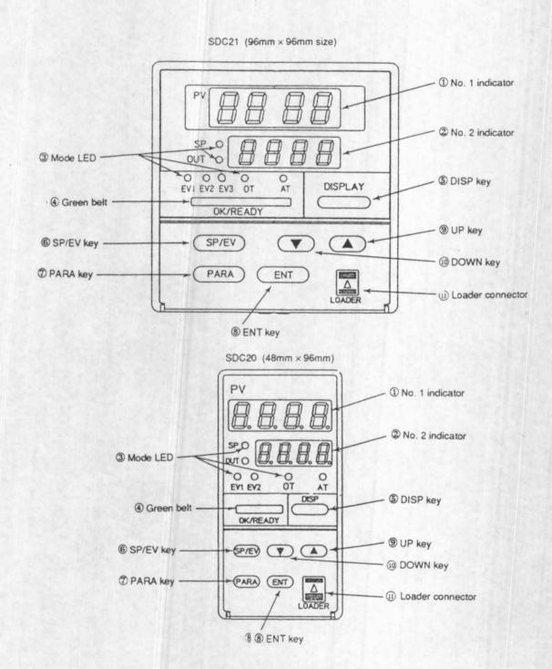
Note: Mode LEDs 3 are called SP LED, OUT LED, EV1 LED, EV2 LED, EV3 LED, OT LED, and AT LED, respectively.
