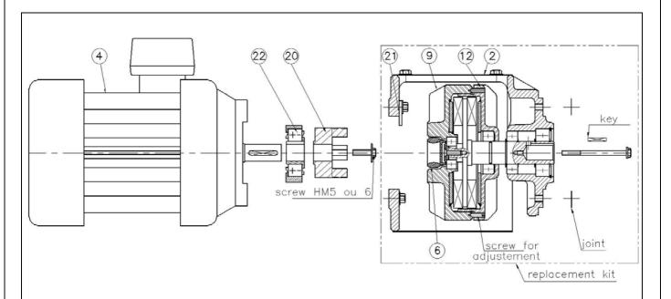
NUTS and BOLTS are assembled using LOCTITE thread-locking product 243
