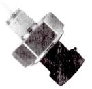
The Model S85 is an active device which is designed to give an alarm signal if fluid falls below a preset level. It will only signal an alarm after a few seconds of low level to eliminate false alarms due to turbulence.
