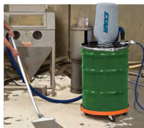
Sand that covers the floor around a sand blaster is quickly vacuumed into the drum using the rugged floor tool.
