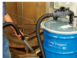
Chip Trapper filters out solids from parts washer fluids.
