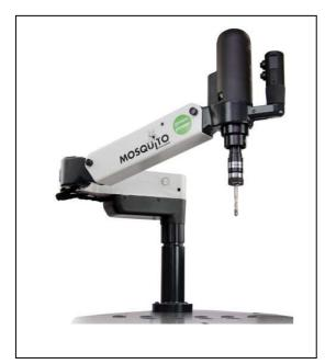
The machine itself consists of a radial arm joint to a tilting arm balanced by means of a pneumatic spring. The head member and the electric motor find themselves at the end of the tilting arm and is adapt to always move at right angle with respect to its working area.
