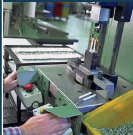
Latest technology at work: the injection molding plant at Beru's Neuhaus-Schierschnitz factory also enables complex ceramic body geometries to be created. Undercuts can also be produced.
