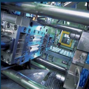
Latest technology at work: the injection molding plant at Beru's Neuhaus-Schierschnitz factory also enables complex ceramic body geometries to be created. Undercuts can also be produced.
