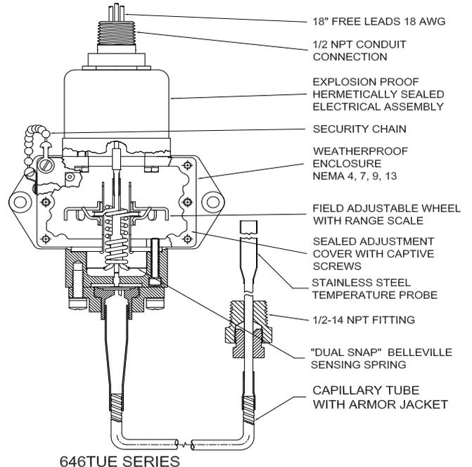
**FIELD SETTING:** Open access cover. Adjust wheel as illustrated. Clockwise to increase settings. Counterclockwise to decrease settings.
