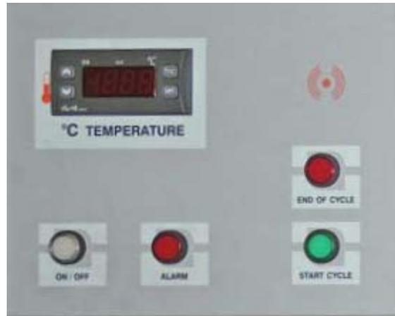
The control system of PLASMA FROST is quite basic and cannot keep track of any freezing data such as the barcode ID of the bags or the date and time of freezing. For top performing plasma freezers with complete data management, computer interface, handling of barcode labels and/or RFID read/write Tags, please refer to the models [PLASMAFROST iTem](#).
