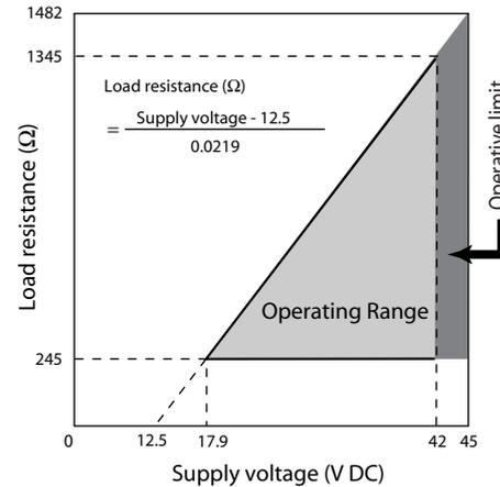
Figure 5 Supply voltage vs. load resistance characteristics
