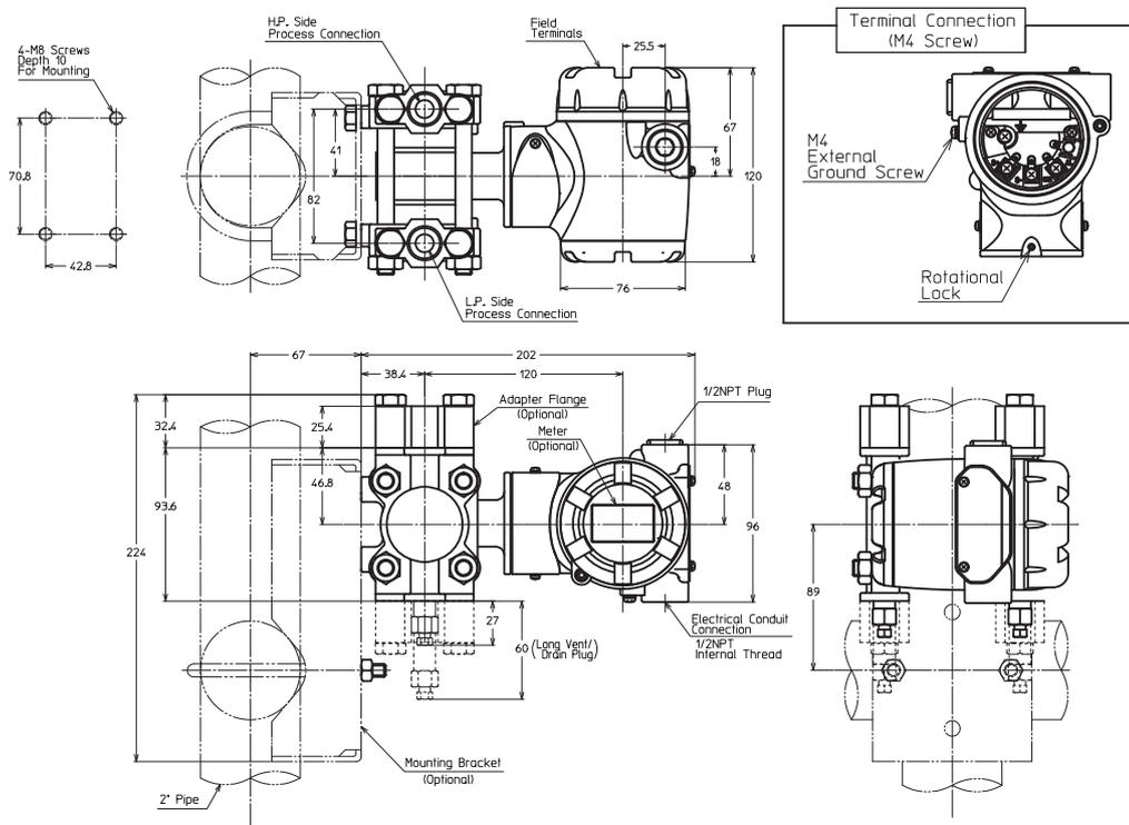
GTX 31D/41D (Material (Meter body cover, Vent/Drain plugs: PVC)
