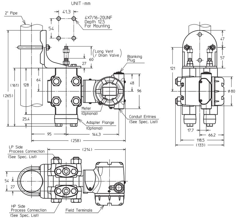
**Model GTX 31D/41D (Material (center body): Tantalum, 316L SST)**
