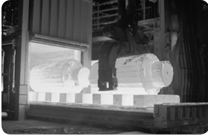
Metallurgical industry: forging furnace
