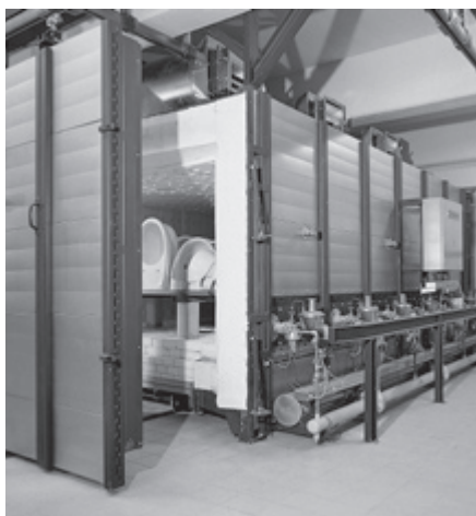
Intermittent shuttle kiln in the ceramics industry
