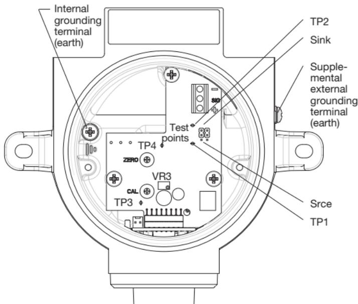
Diagram 14: **Xgard** Type 6 PCB layout
