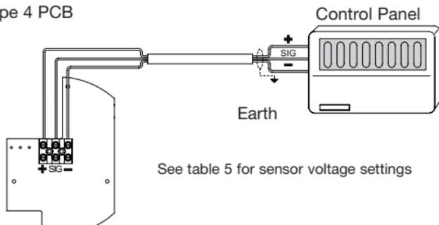
Diagram 11: Xgard Type 4 electrical connections
