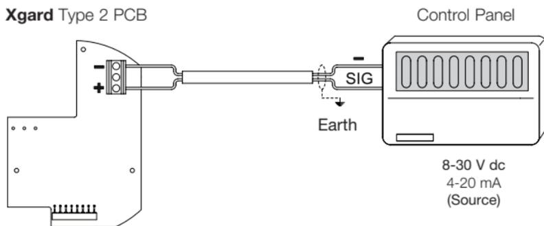
Diagram 7: **Xgard** Type 2 electrical connections
