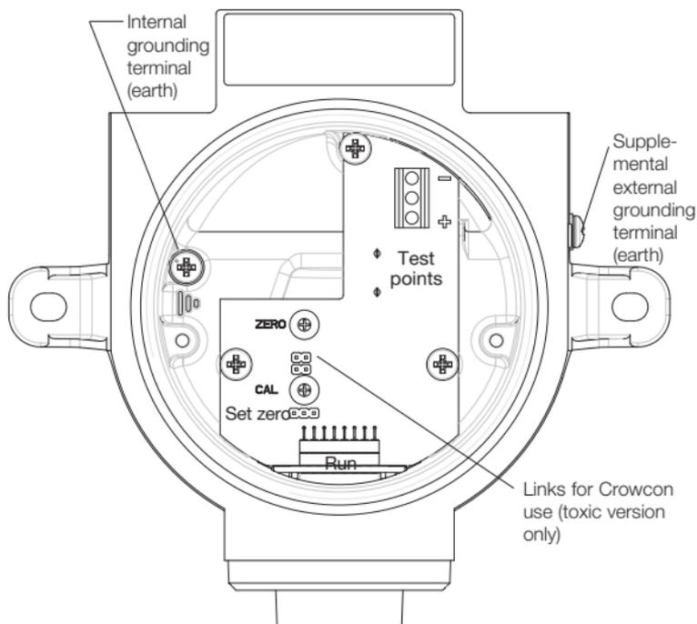
Diagram 4: **Xgard** Type 1 PCB layout
