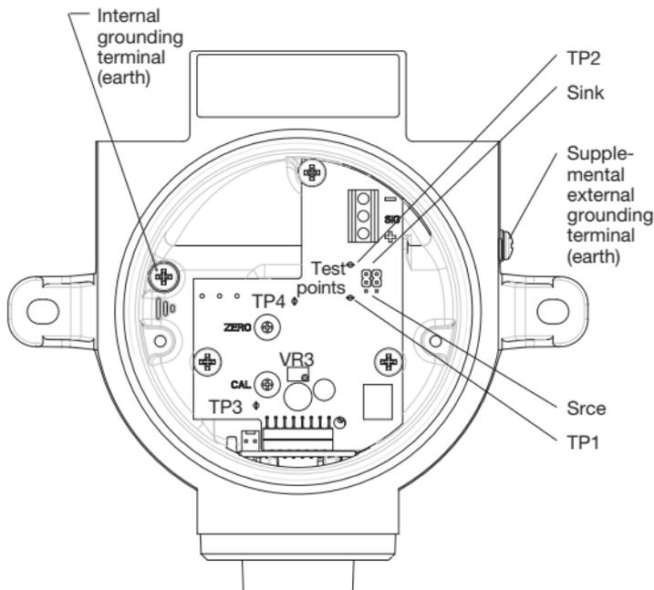
Diagram 12: **Xgard** Type 5 PCB layout
