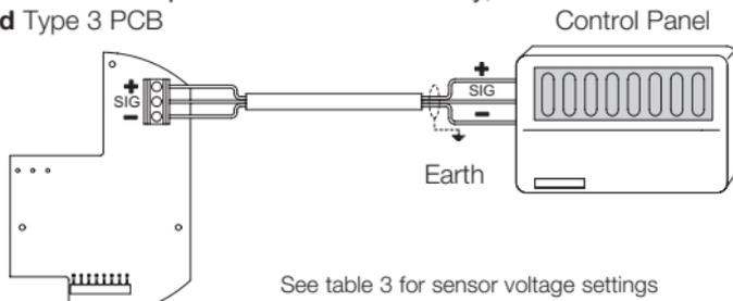
Diagram 9: Xgard Type 3 electrical connections
