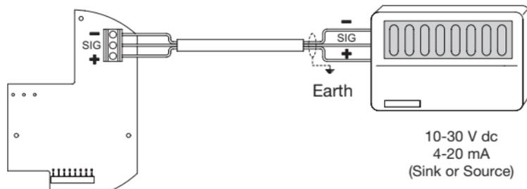
Diagram 13: **Xgard** Type 5 electrical connections
