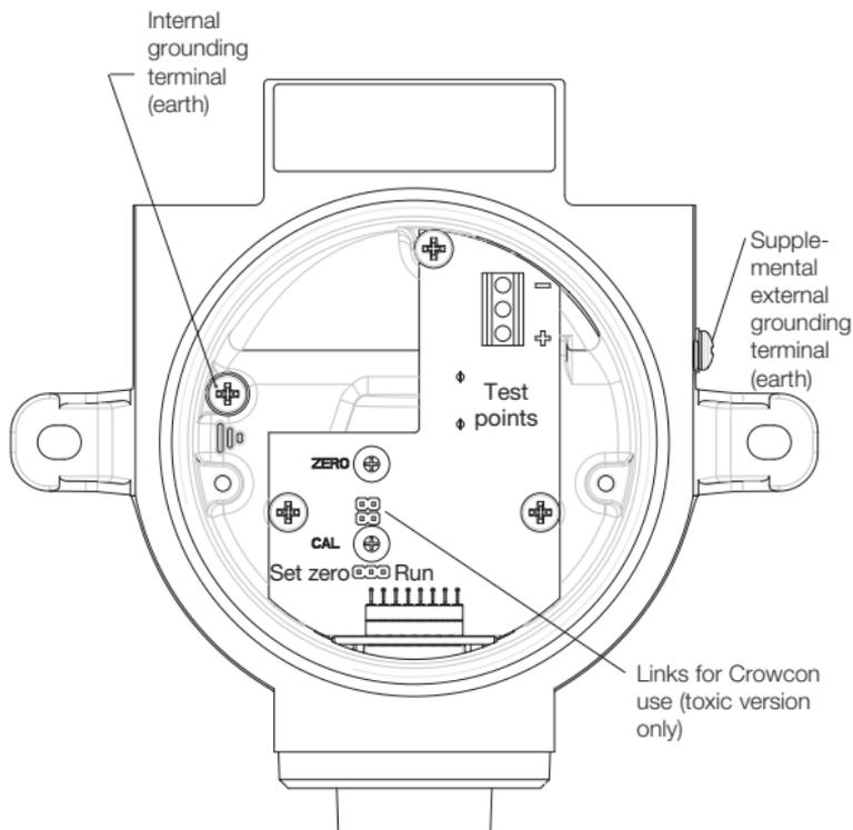
Diagram 6: **Xgard** Type 2 PCB layout
