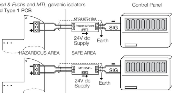
Diagram 5: **Xgard** Type 1 electrical connections
