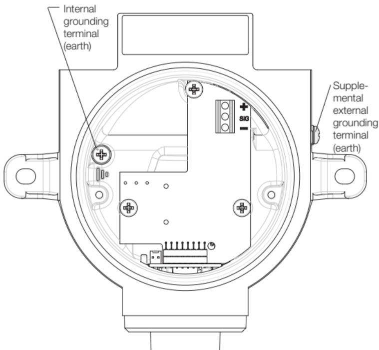
Diagram 8: **Xgard** Type 3 PCB layout
