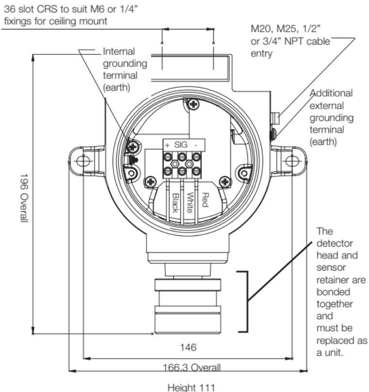
Diagram 10: **Xgard** Type 4 dimensioned view
