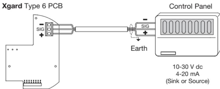
Diagram 15: **Xgard** Type 6 electrical connections
