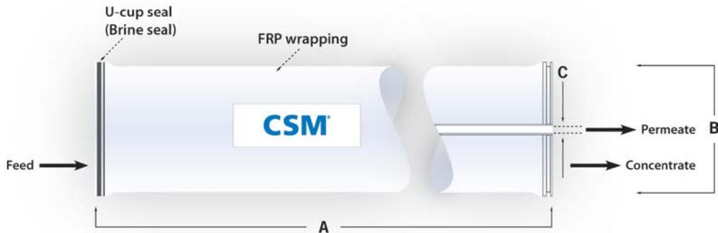
1. Each membrane element comes with one brine seal, one interconnector (coupler) and two o-rings.
