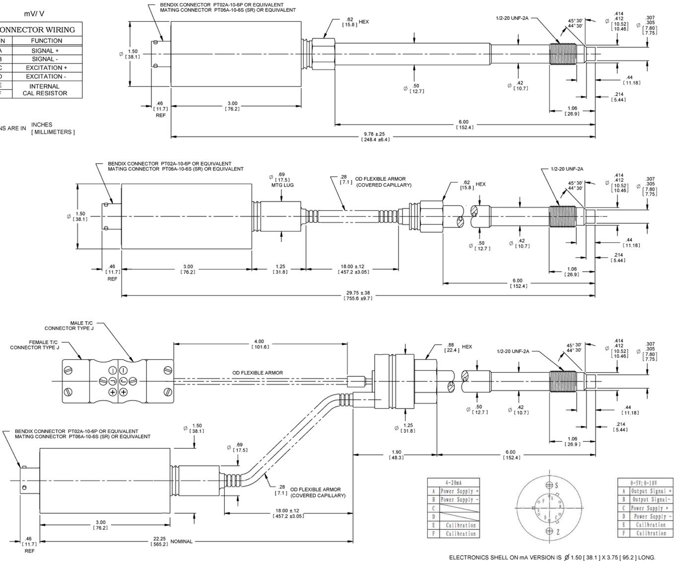
ELECTRONICS SHELL ON mA VERSION IS  $\varnothing$  1.50 [38.1] X 3.75 [95.2] LONG.
