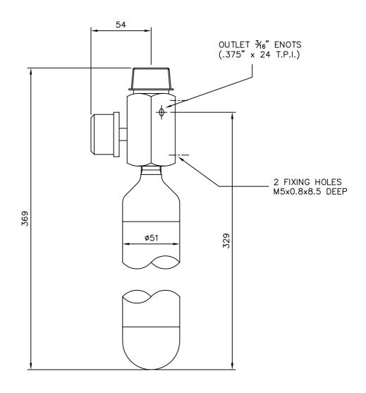
DRY NITROGEN TO 65 BAR AT 20°C CHARGE:
