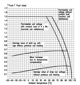
Permissible coil voltages and pick-up and drop-out characteristics at various ambient temperatures.
