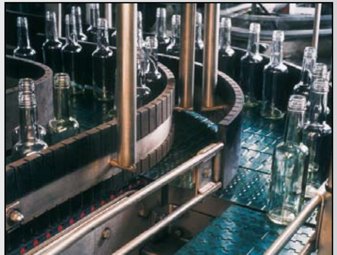
GLASS BOTTLE MANUFACTURING ON 1005 FLAT TOP BELT
