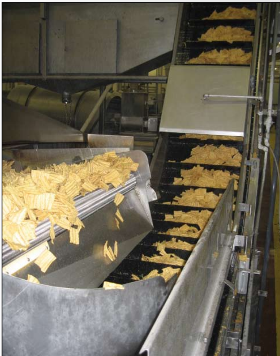
INCLINED CONVEYOR FOR CHIPS FTR2015 BELT
