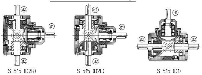
D2R = Kegelrad oben D2L = Kegelrad unten D2R = bevel gear at top D2L = Kegelrad at bottom
