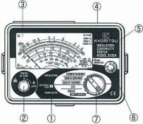
**①METER MOVEMENT ZERO ADJUST 2TEST BUTTON 3SCALE PLATE** (4) INPUT CONNECTOR **5LIVE CIRCUIT LAMP ©OHMS ZERO ADJUST PRANGE SELECTOR SWITCH**
