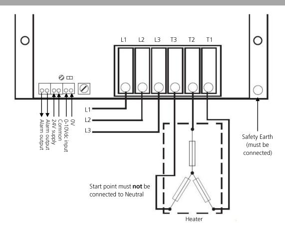
NOTE: It is imperative that the power connections are fully tightened, without excessive force, and ensure the maximum area of cable is in contact with the terminals.
