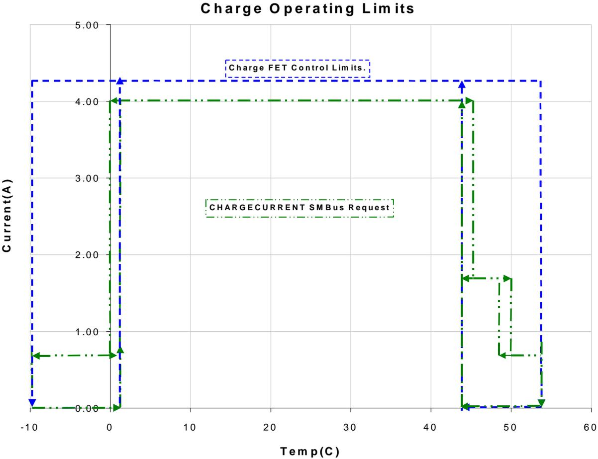
NOTE: If not charging & temperature > 45C then the battery enters Charge-Inhibit where ChargingCurrent() = 0 & ChargeVoltage() = 0 until temperature  $\leq 44C$
