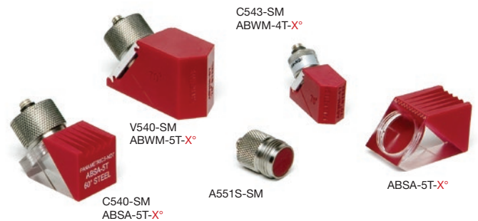
Miniature angle beam transducers and wedges are used primarily for testing of weld integrity. Their design allows them to be easily scanned back and forth and provides a short approach distance.
