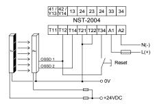
$\hbox{2-channel protection door monitoring without short circuit protection}$
