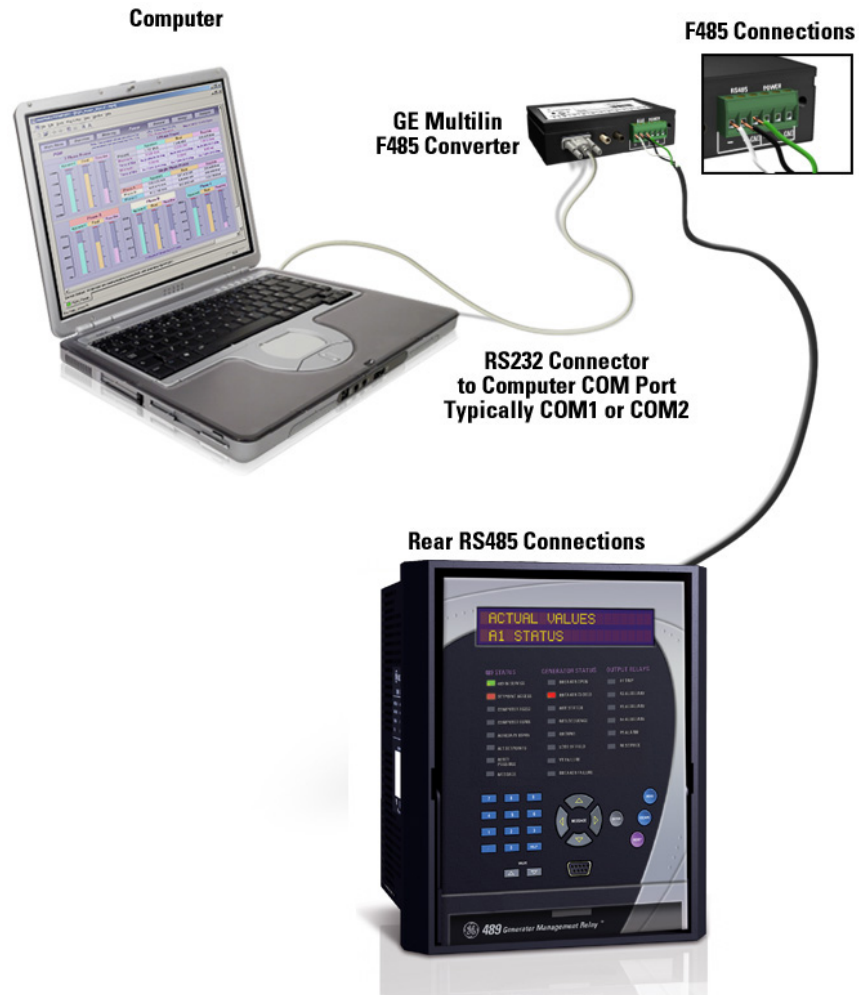
FIGURE 4-3: Communications using Rear RS485 Port
