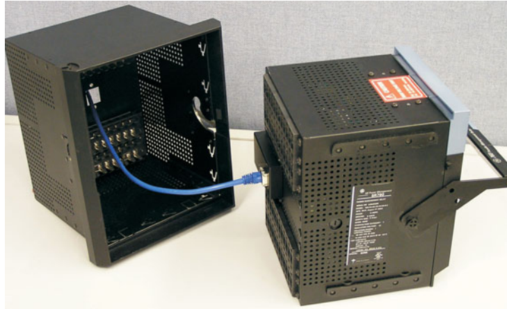
FIGURE 3-8: Ethernet Cable Connection
