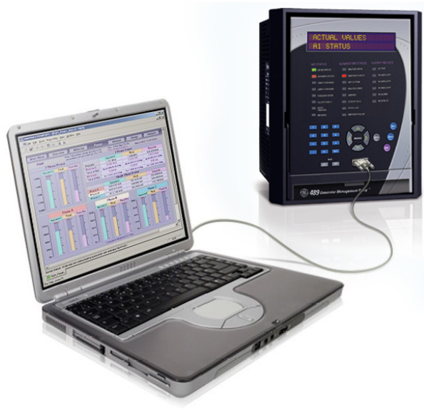
FIGURE 4-2: Communications using The Front RS232 Port
